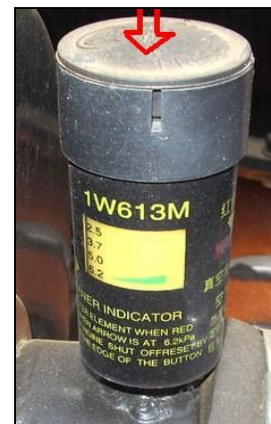
Service Indicator Press the Top to reset
