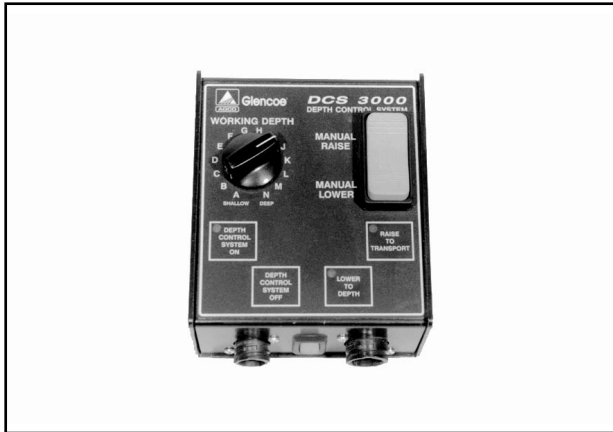
Figure 4-37 Depth Control System Console
