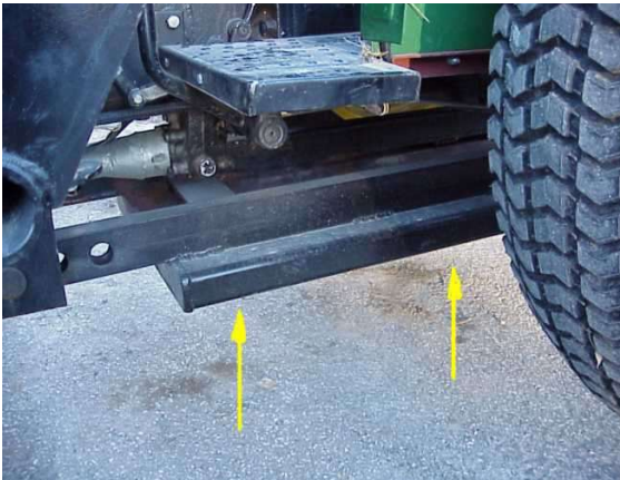
Figure 40. Hoe Frame showing heavy reinforcement
