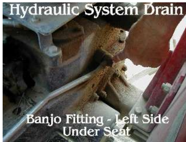
Figure 35. Hydraulic System Oil Drain
