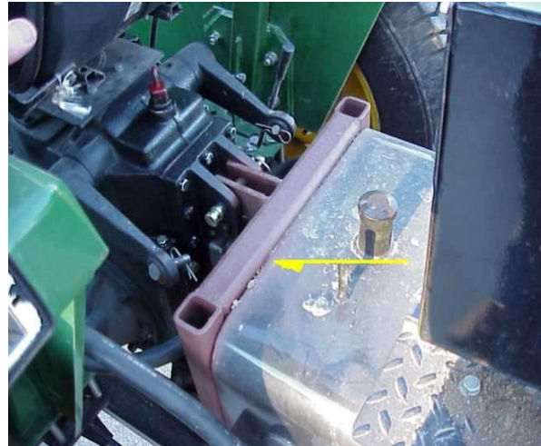
Figure 44. Hoe frame top link stabilizer
