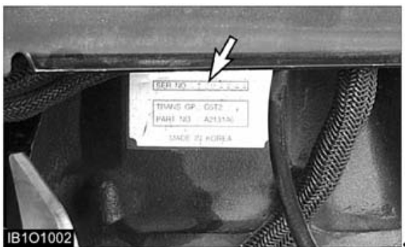
Power Shift Transmission Serial Number
