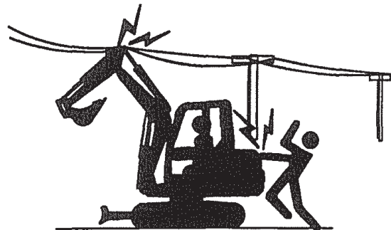
Electrical shock / electrocution
