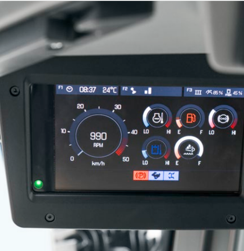
The 7-inch LCD display shows all of the important data.
