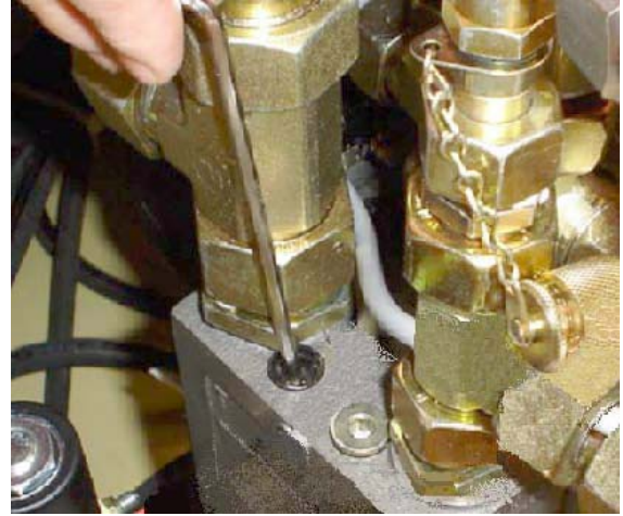
Figure 4-39. Proportional Valve Pressure Adjustment
