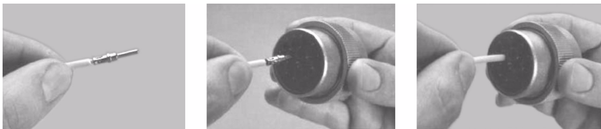
Figure 6-14. HD/HDP Contact Installation
