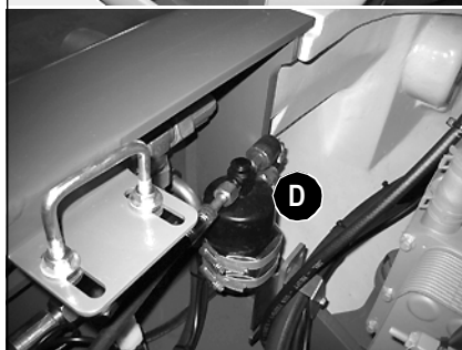
Fig. 186: Air conditioning: heat exchanger, dehumidifier
