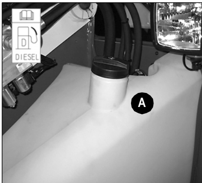
Fig. 155: Main tank fuel filler inlet
