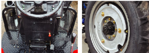
Rear Wheel Track Stepless Adjustable
