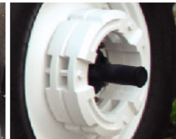
Rear Wheel Track Stepless Adjustable
