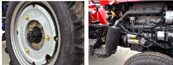
Rear Wheel Track Stepless Adjustable
