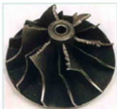
Compressor impeller damaged by particles
