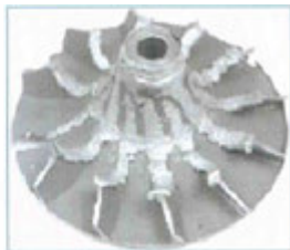
Compressor impeller damaged by solid objects
