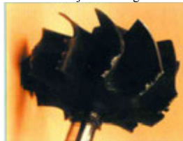
Turbine impeller damaged by particles
