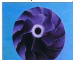
Compressor impeller damaged by dust
