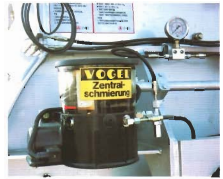
3 Lubricating Oil Pump
