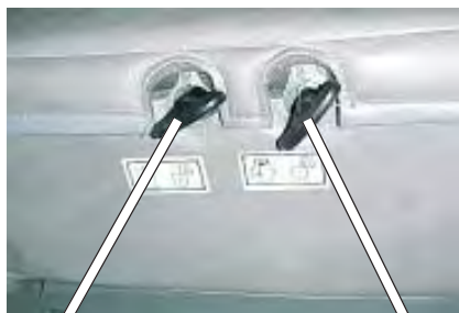
Pict.: Bowdenzug - operation inside the cabine
