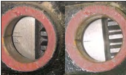
Fig. 11: Top dead centre indentation and 10° before top dead centre
