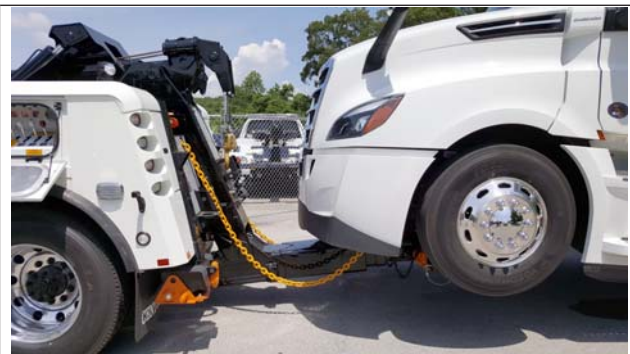
Fig. 23.14, Final Towing Position
