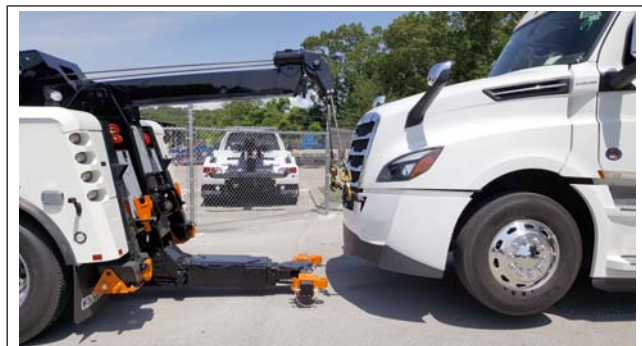
Fig. 23.7, Tow Cables Connected to the Tow Hooks
