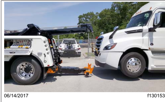
Fig. 23.10, Backing the Tow Truck with Lift Adaptors on the Crossbar
