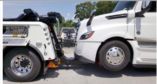
Fig. 23.14, Final Towing Position
