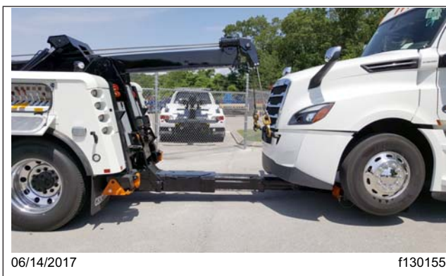
Fig. 23.12, Stinger with Lift Adaptors Under the Axle (tow truck shown)
