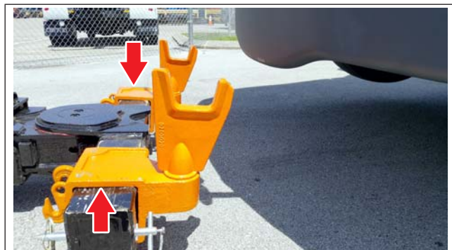
Fig. 23.8, Moving the Stinger and Crossbar Under the Bumper
