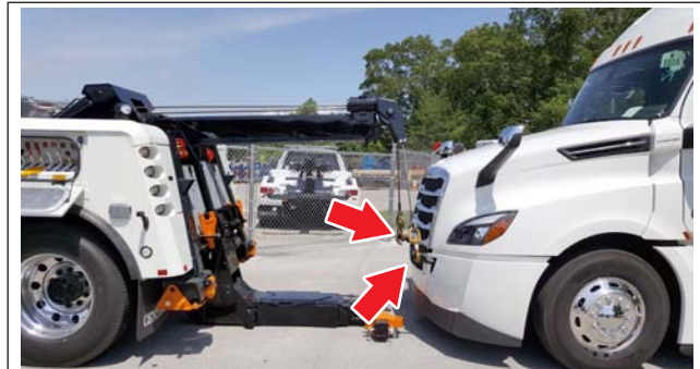
Fig. 23.7, Tow Cables Connected to the Tow Hooks
