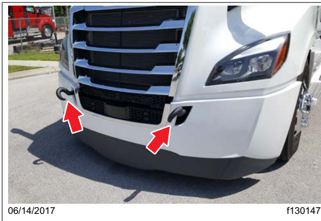
Fig. 23.4, Tow Hooks Installed, Facing Down
