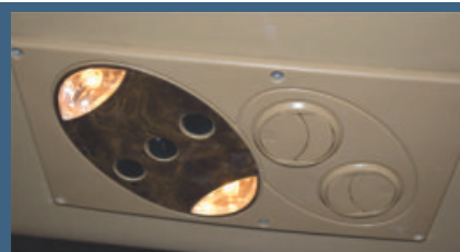
Individual AC Louvers & Reading Lamps
