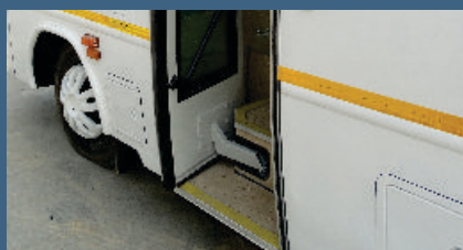
Low Footstep Entry with Driver Controlled Electronic Door
