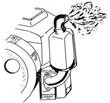
Fig.8 Engine exhausting black smoke
