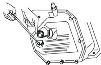
Fig.3Checking engine oil
