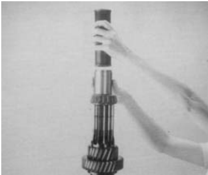
7. Using the proper size bearing driver, install the countershaft rear bearing on the countershaft rear. Make sure the bearing is seated against the countershaft.
