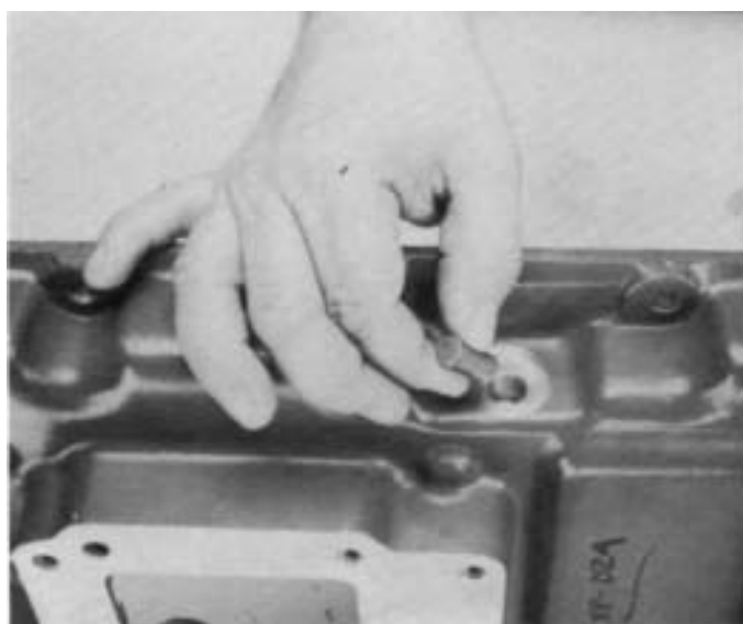
12. Install the reverse light switch pin in the shift bar housing.
