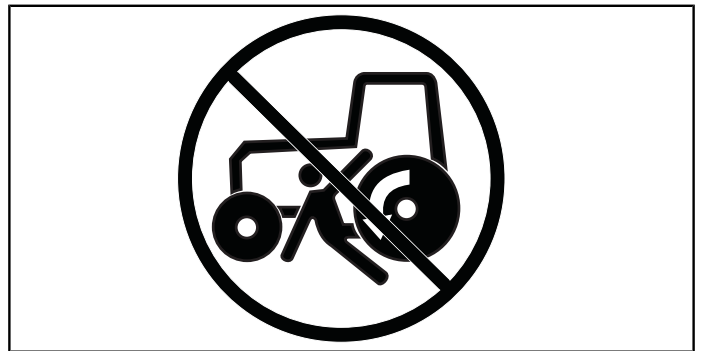
Fig. 18 Only operate the machine when sitting in the operator's seat.
