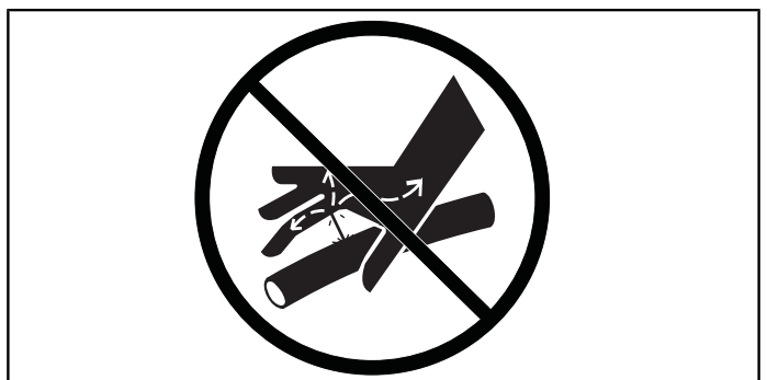
Fig. 87 NEVER use fingers or hands to detect leaks.
