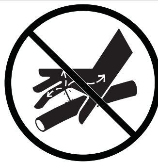
Fig. 14 NEVER use fingers or hands to detect leaks.
