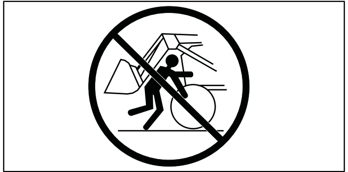
Fig. 85 Never stand between the front of the loader and the cross-tube on the loader.
