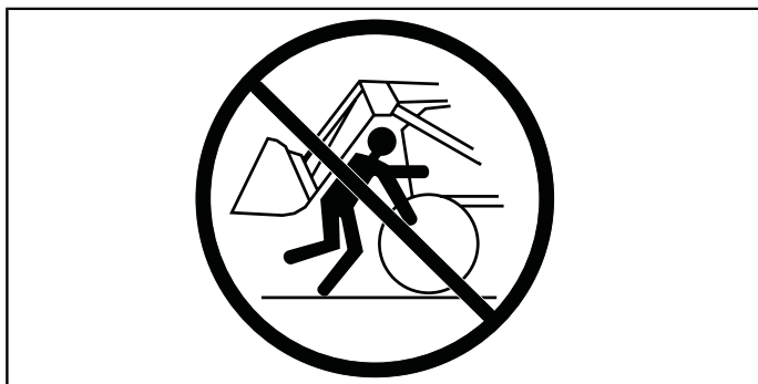
Fig. 25 Do NOT stand, walk or work under a raised loader.
