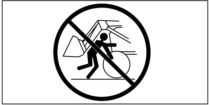
Fig. 58 Do NOT stand, walk or work under a raised loader.
