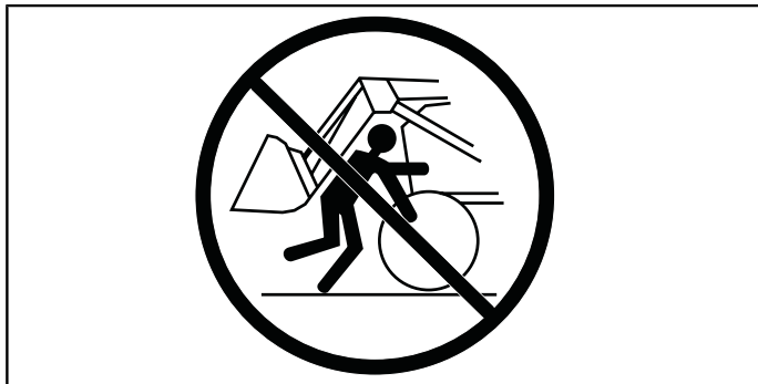
Fig. 26 Never stand between the front of the tractor and the loader's cross tube.
