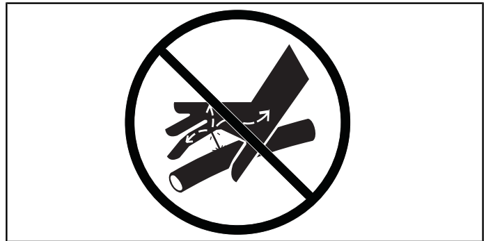
Fig. 39 NEVER use fingers or hands to detect leaks.
