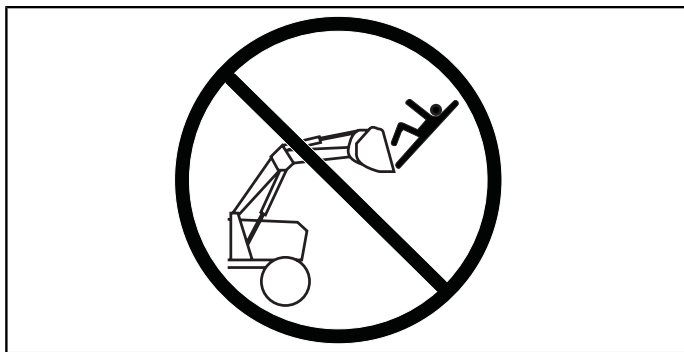
Fig. 23 Do NOT use the loader or the implement/bucket as a work platform.
