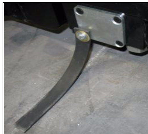
Figure 5-2 Static Discharge Straps
