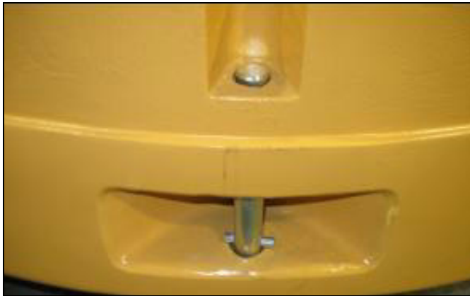
Figure 2-3: Tow Pin Used for Towing
