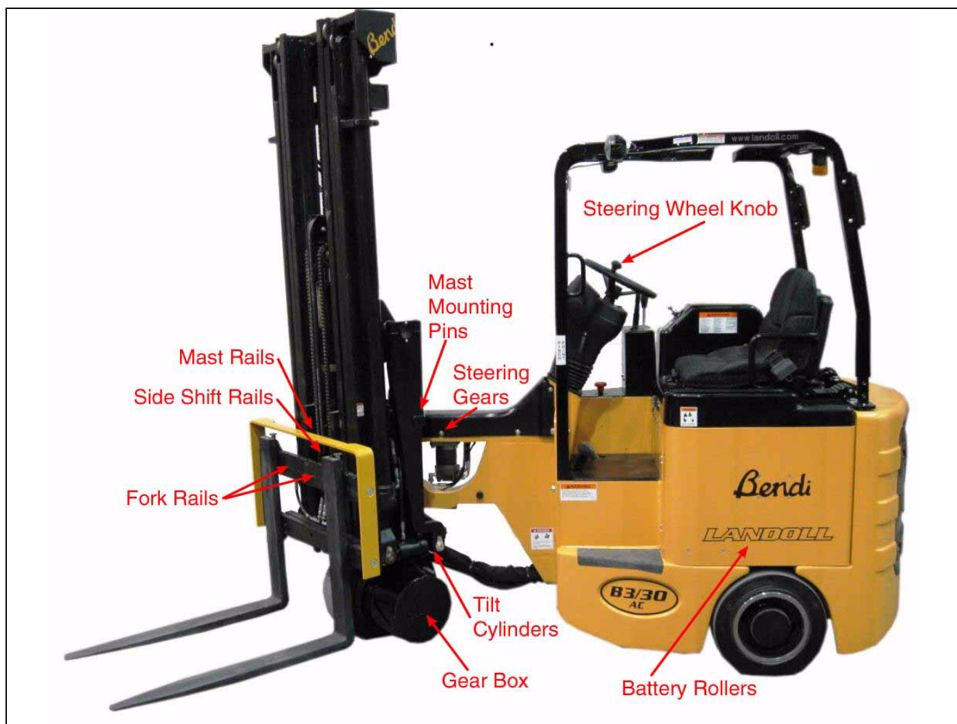
Figure 5-8: Lubrication Points
