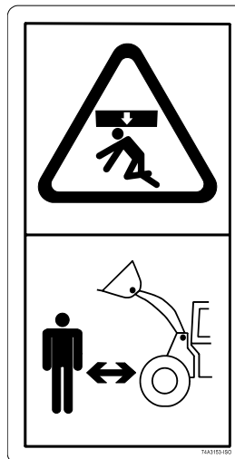
Fig. 2 DANGER DECAL (Located on the arm) CRUSH HAZARD. Keep away from raised loader arm or bucket.
