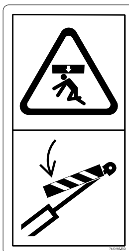
Fig. 3 DANGER DECAL (Located on the arm or arm cylinder) CRUSH HAZARD. Install arm support before maintenance or repair with loader arm raised.
