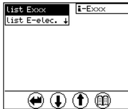
Fig. 3-22 Menu "i-errors" - operating faults and electrical system errors
