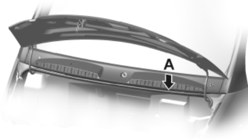
Fig. 1.2. A — Location of Cab Identification Number
