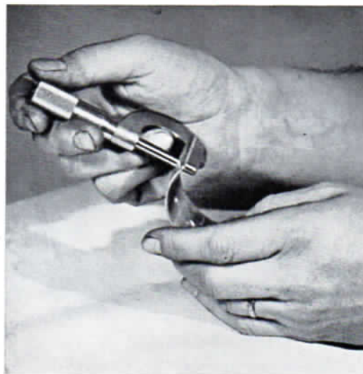
FIG. 26 CHECKING CONNECTING ROD BEARINGS WITH BALL MICROMETERS
