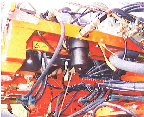
Figure 1. Anti extrusion ring installation
