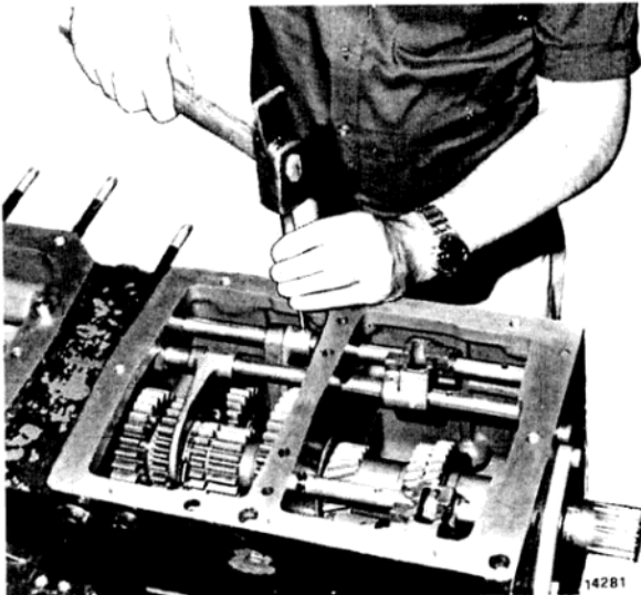
Removing transmission and splitter shifter fork and gate roll pins.
