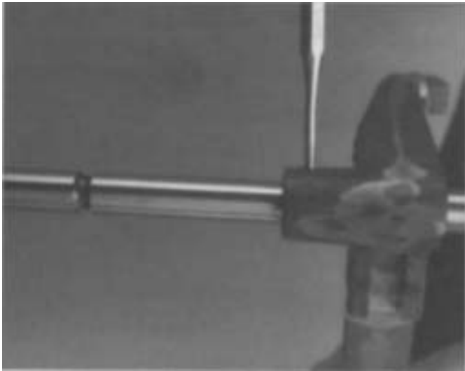
11. If it is necessary to replace yoke or shift blocks, secure shift rail in a vice equipped with brass jaws or wood blocks. Drive the roll pin from yoke and yoke bar as shown.
