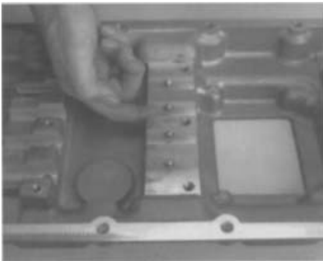
8. Install interlock balls in the shift bar housing, position two interlock balls in the first-second crossbore, third-fourth crossbore, and the fifth-sixth crossbore.
