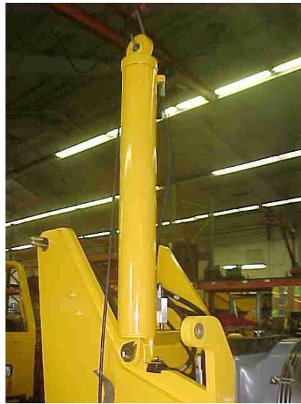
LIFT CYLINDER ON HOIST
