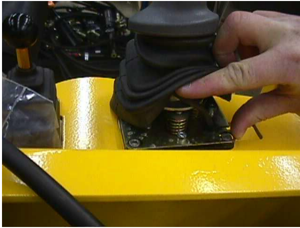
MOUNTING BRACKET CAPSCREWS
