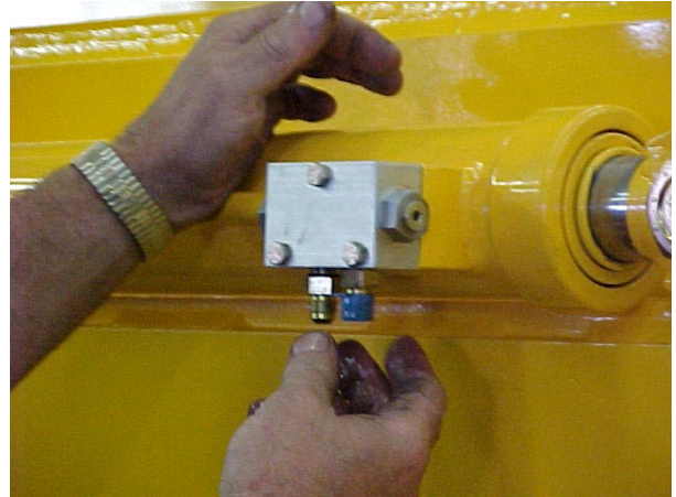
PROTECTIVE CAPS ON VALVE BLOCK.
