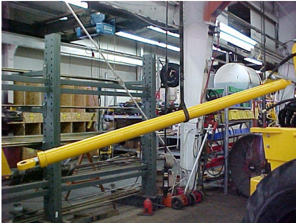
LIFTING THE CYLINDER INTO POSITION.
