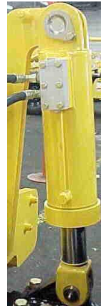
FULLY INSTALLED SWAY CYLINDER
