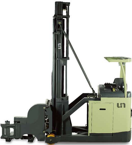
VNA MAN-DOWN capacity 1,300kg
