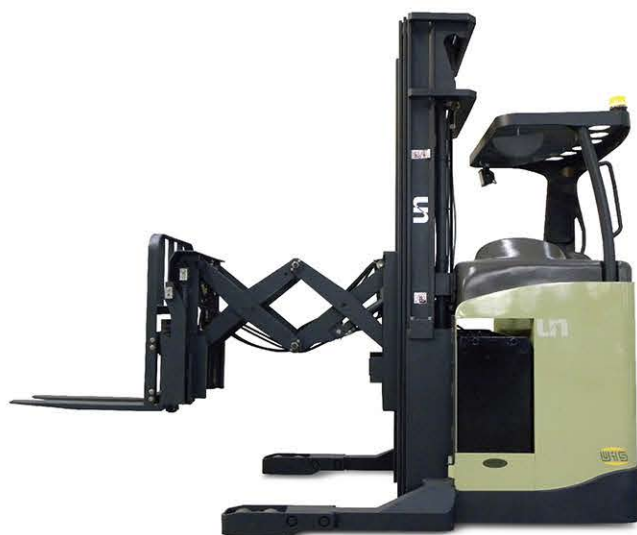
Double Deep Reach Truck capacity 1,500kg
