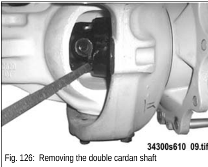
Fig. 126: Removing the double cardan shaft
