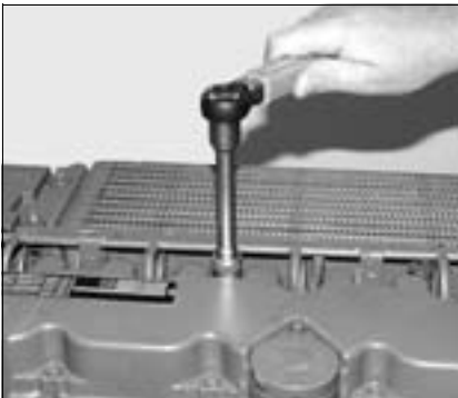
Fig. 53: Mounting the cylinder-head cover
