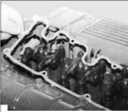
Fig. 52: Placing the cylinder-head cover gasket
