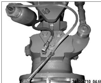
Fig. 135: Bleeding the brakes
