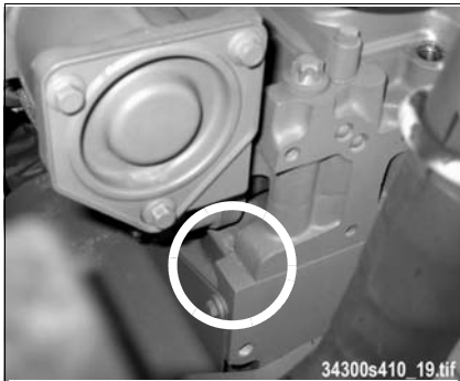
Fig. 72: Determining the cylinder-head gasket
