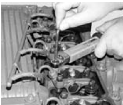
Fig. 51: Setting valve tip clearance
