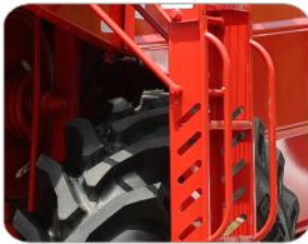
Ladder cover with sheet for safety purpose
