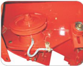
Cutting blade driven thru. Gear mechanism
