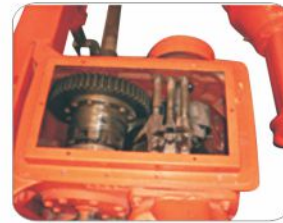
Heavy duty gearbox with five speeds Collar shift gears
