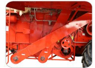
Stainless steel sheet used for long life of parts which are subjected to more wearing like elevators. Used UCF bearing is widely appreciated for durability and long serviceability
