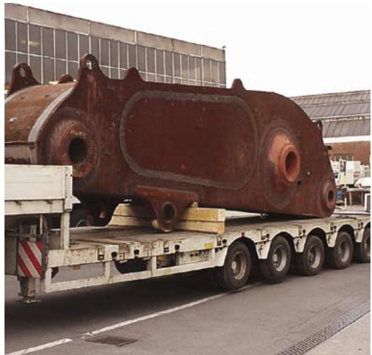
Each boom and stick is stress relieved after welding.
