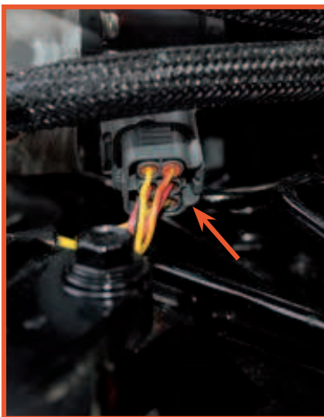
IP67 watertight electrical connections.
