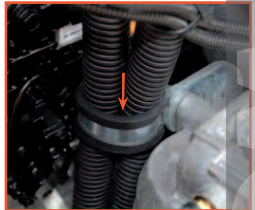
Anti-wear supports for corrugated cable sheaths.
