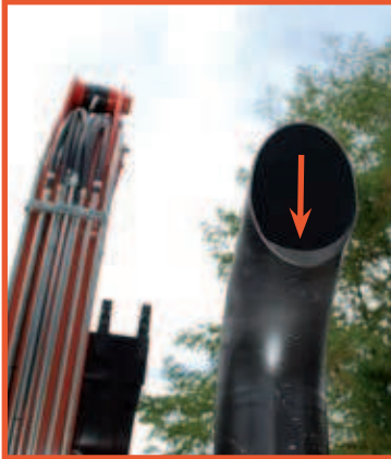
Waterproof membrane that prevents rust from forming in the exhaust pipe.
