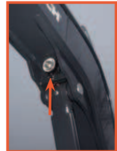
2 lights for the work area on the turret and 1 protected light under the boom.
