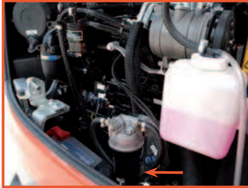
Sensor that indicates by means of a light if there is water in the filter.
