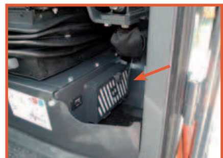
Compartment inside cab for storing items and air circulation filter.
