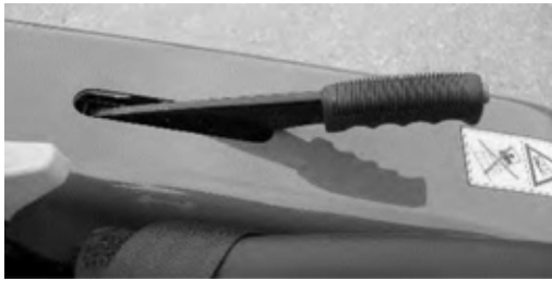
The parking brake is released in position "A"
