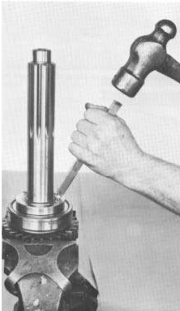
4. Relieve drive gear bearing nut at points where peened into shaft.
