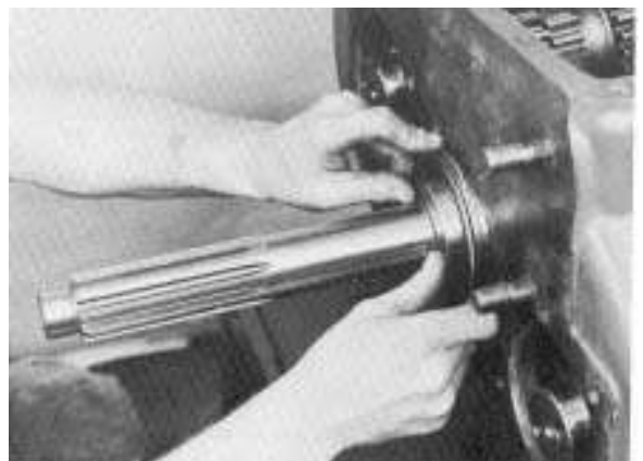
10. Install snap ring on drive gear bearing.
