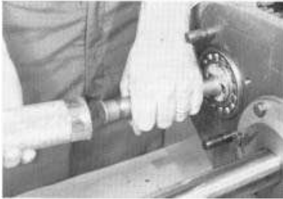
3. Move countershaft to the rear as far as possible, this will move rear bearing to the rear and partially unseat front bearing.
