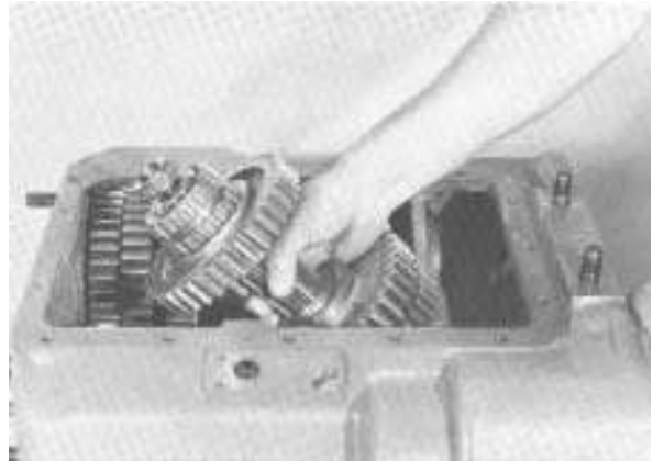
21. From inside case, insert rear of mainshaft through rear bearing bore; lower assembly into position.
