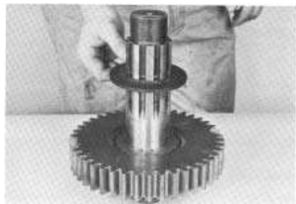
5. Install rear washer on shaft.
