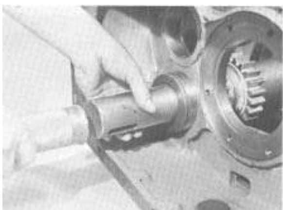
3. Install rear bearing on left countershaft and into case bore.
