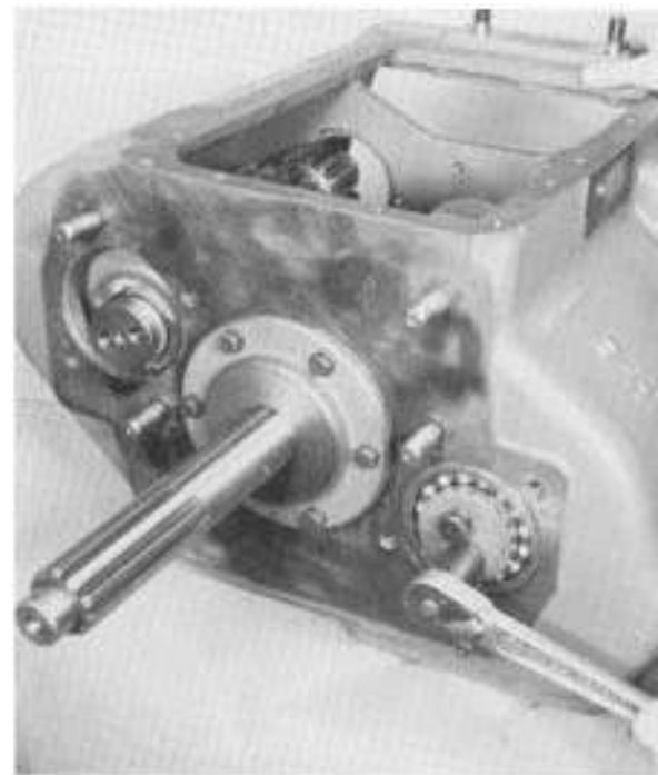
7. Remove bearings from left countershaft in the same manner as bearings were removed from right countershaft.
