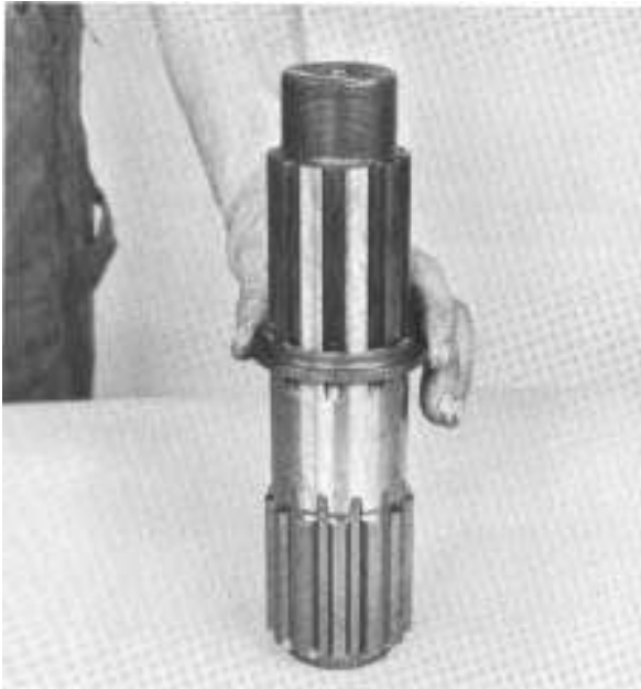
1. Install stepped washer on auxiliary mainshaft.
