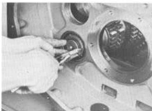
5. Install the snap ring on rear of left countershaft.
