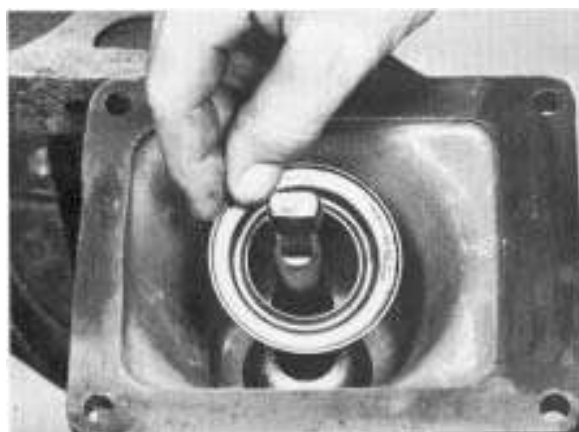
3. Place the tension spring washer in housing.
