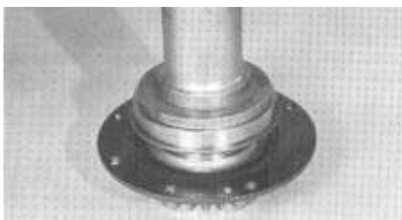
2. Press bearing on drive gear
