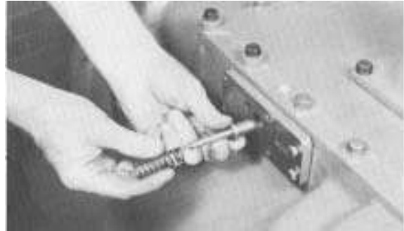
9. Remove spring and actuating pin.
