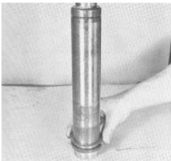
1. Install the countershaft front spacer.
