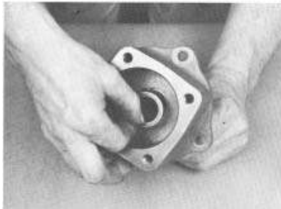
2. Install washer in shift cylinder against O-ring.
