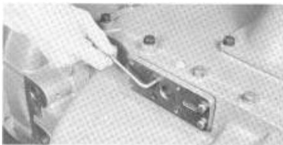
2. Install gasket and the air valve adapter plate. This takes two x-8-425 caoscrews, and two x-8-410 capscsrews with x-3-400 washers. Make sure adapter plate is perfectly aligned with bore in case.
