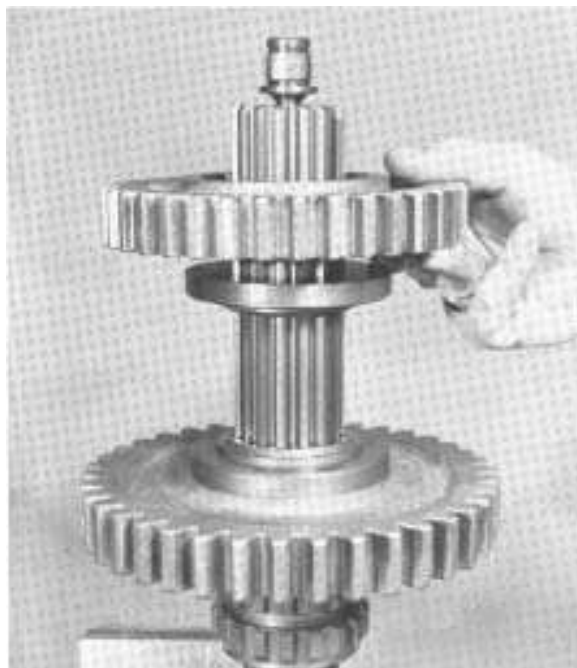
11. Install the 2nd speed gear , clutching teeth up.
