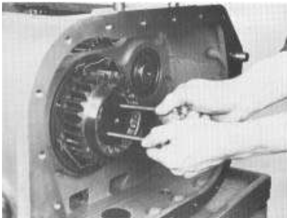
2. Insert puller screws and remove quill support plate from gear.
