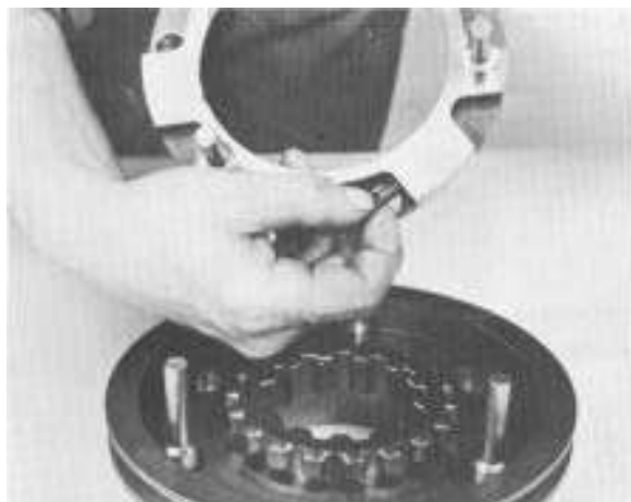
2. Install the three springs in direct synchronizer.
