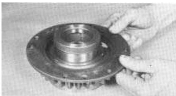
1. Place retainer ring on auxiliary drive gear.
