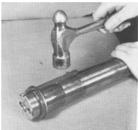
2. Install the front key in countershaft.
