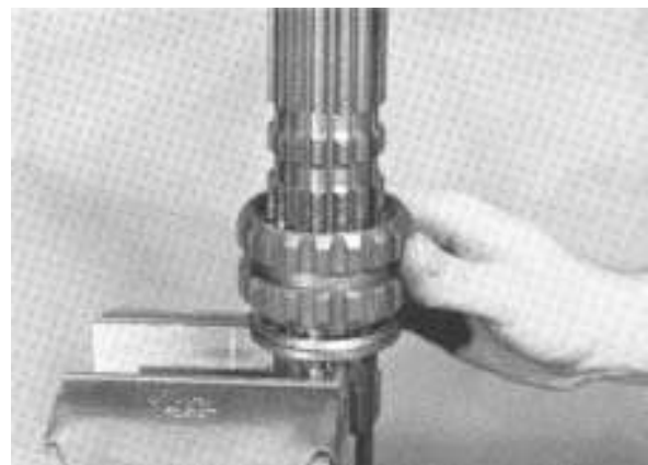
3. Install the first-reverse sliding clutch on shaft.
