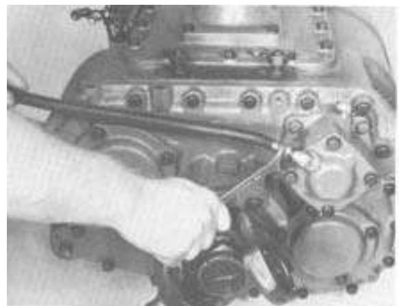
6. Remove air lines from range shift cylinder.
