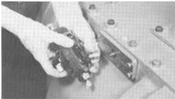
8. Remove alignment sleeve from air valve.
