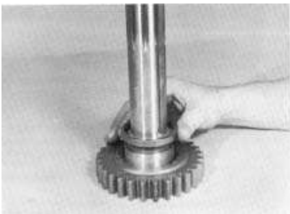
3. Install spacer on shaft.
