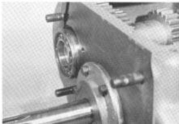
5. Front bearing snap ring will be exposed when countershaft is moved forward as shown in step 4.
