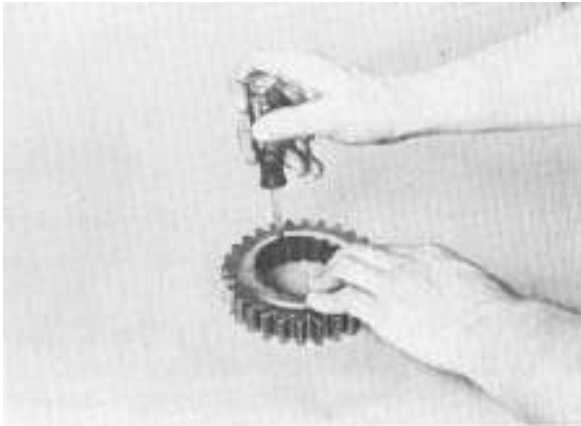
1. Install snap ring in ID of drive gear.
