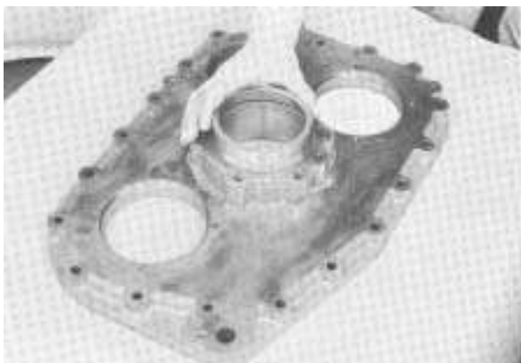
8. Place front cup of bearing partially in rear bore, taper to the inside.
