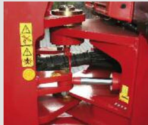
The diameter of the articulation joints is 80 mm.
