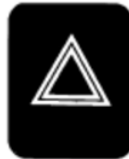
Hazard Flasher Light Switch PART NO: 390380770 LOCATION: Right Side of Dash
