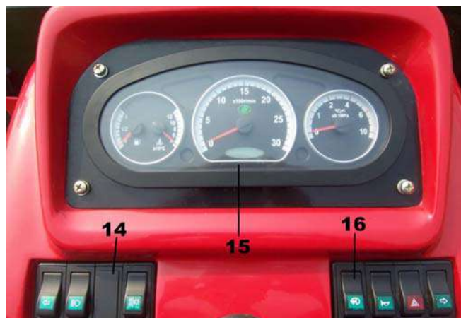
Fig.4-4 combined gauges and switches
