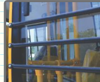
Windows Guard-rails for Children's Safety
