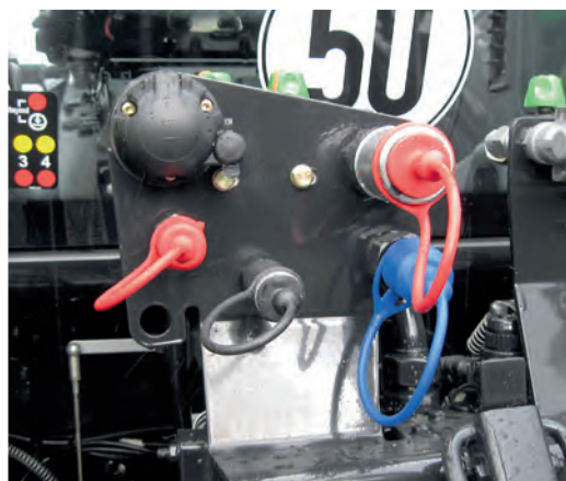
To order the Agrottron M can be fitted with Power-Beyond connectors for the direct connection of third-party devices.
