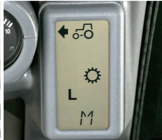
Everything in view: The central display of the Powershift stages in the A-strut.
