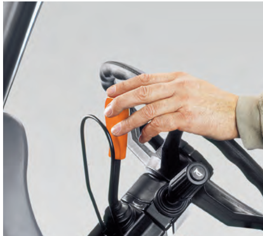
Changing the direction of travel without actuating the clutch: the standard Powershuttle.
