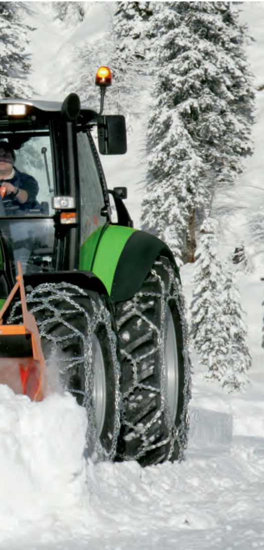
Changing the direction of travel without actuating the clutch: the standard Powershuttle.
