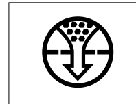
Air cleaner filter contamination warning lamp
