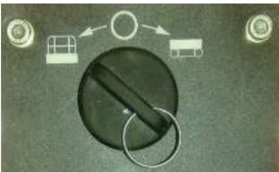
Fig. 22 Chassis control position
