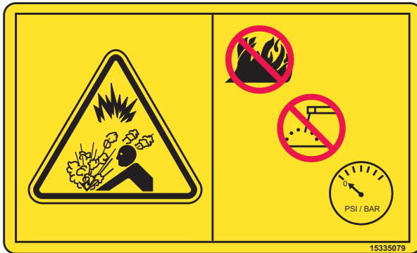
Pressurised Accumulator Warning. Do not weld, keep away from flames. Relieve all pressure before servicing (1893)
