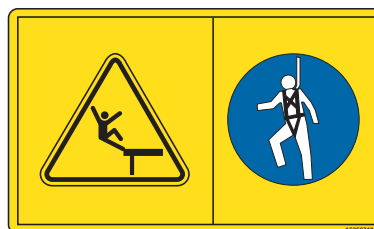
Fall Hazard Warning. Use Safety Harness provided (2219)
