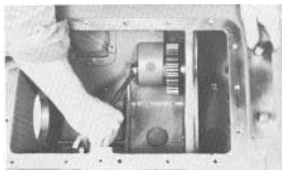
6. Install elastic stop nut and retainer washer on shaft. (if desired the auxiliary countershaft front bearing can now be installed in the right reverse idler bore).
