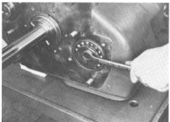
6. Install the bearing retainer plate on front of left countershaft. Tighten and wire securely.
