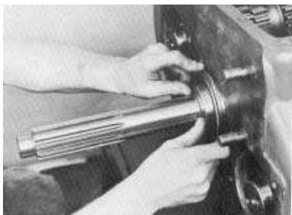
10. Install snap ring on drive gear bearing.
