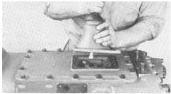
1. Remove gear shift lever housing assembly.
