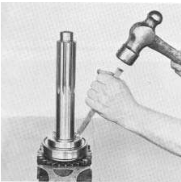
7. Peen nut into the two slots of shaft.
