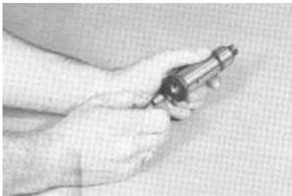
1. Install plug in reverse idler shaft.
