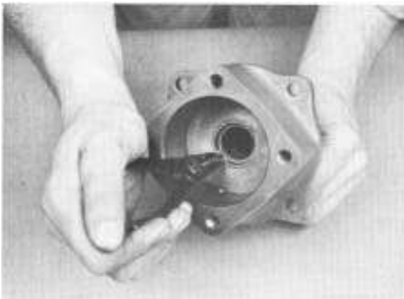
3. Install snap ring in shift cylinder to secure washer and O-ring.
