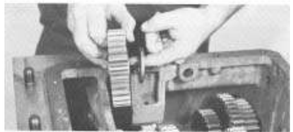
5. Remove reverse idler gear and washer from case.
