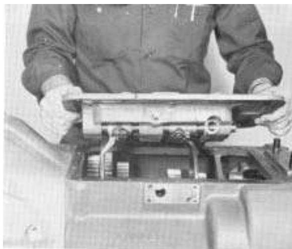
7. Install the shifting bar housing on transmission, fitting yoke forks into slots in sliding clutch gears.
