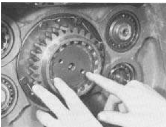
9. Install the rear quill support plate, flat side to the rear.
