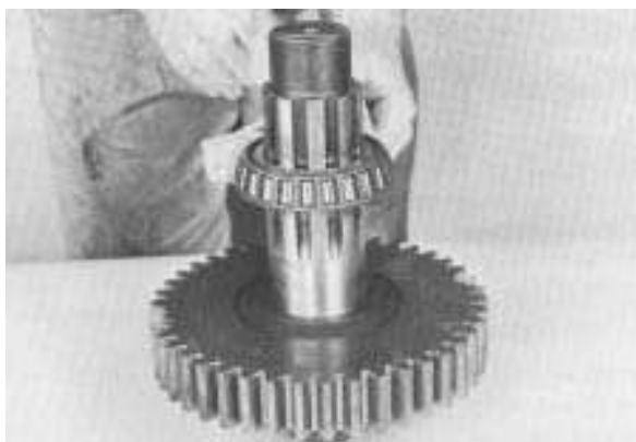
6. Install front cone of rear bearing on shaft; seat against washer. (heating of bearing cones will facilitate installation. Use heat lamps and do not heat over 275 degrees F.
