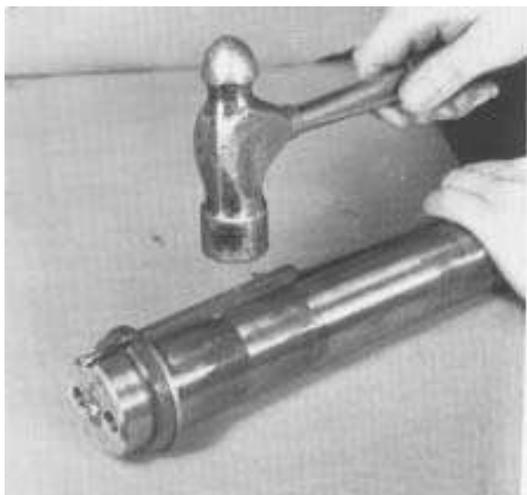
2. Install the front key in countershaft.
