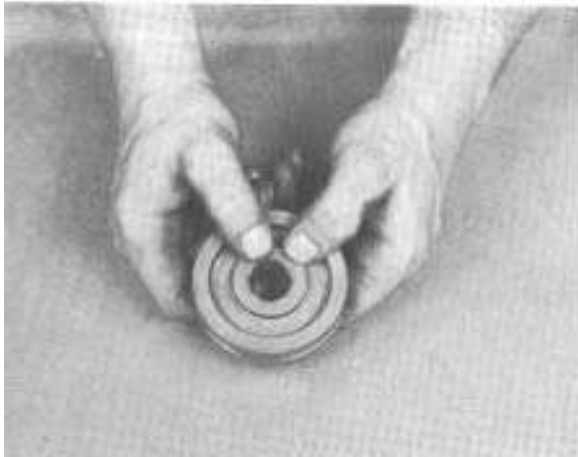
7. Install O-ring in ID of piston.
