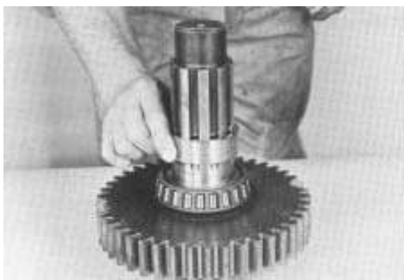
7. Install bearing inner spacer on shaft and against bearing cone.
