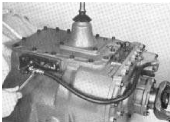
6. Install the high range air line between port in range cylinder cover and rear port in air valve.
