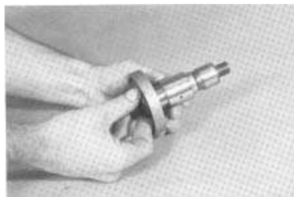
3. Install bearing inner race on shaft and against cup.
