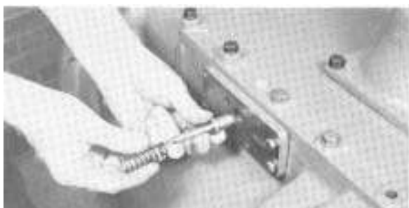
3. Install the actuating pin and spring in bore.
