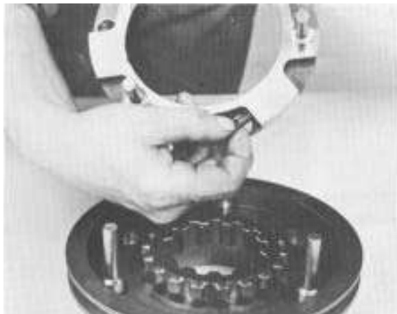
2. Install the three springs in direct synchronizer.
