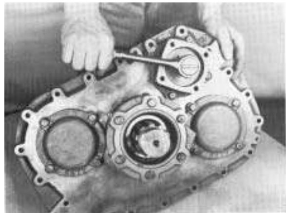
2. Turn nut from air cylinder shifting bar
