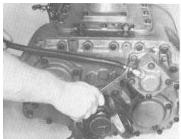
6. Remove air lines from range shift cylinder.
