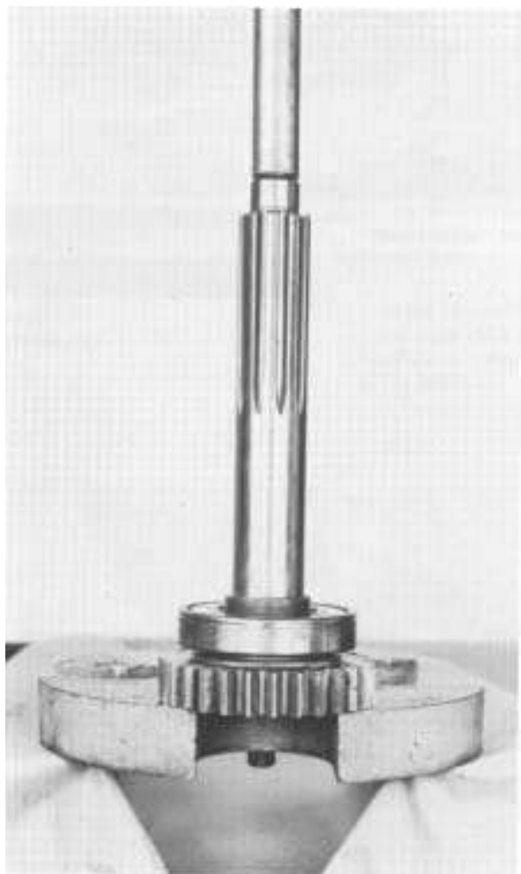
6. press shaft through gear and bearing; Remove snapping from ID of drive gear if necessary.
