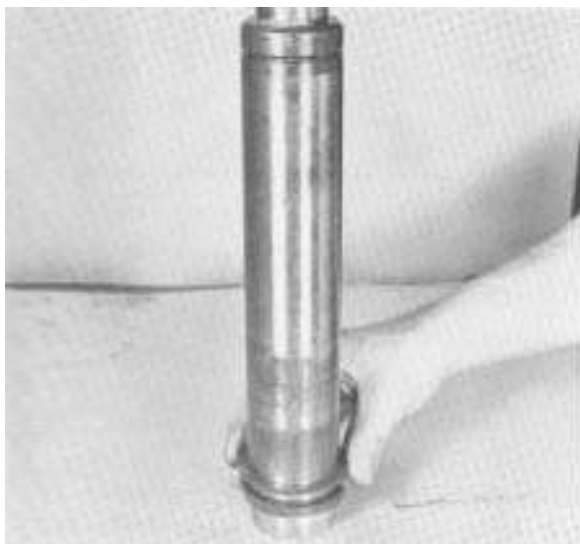
1. Install the countershaft front spacer.
