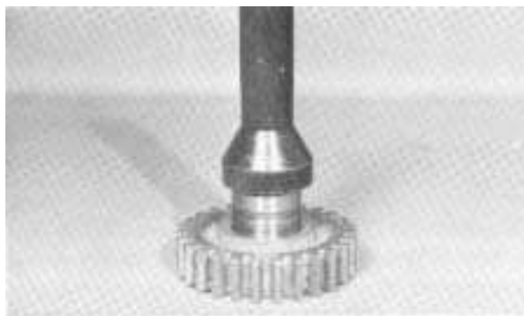
4. Press needle bearing in bore of reverse idler gear.
