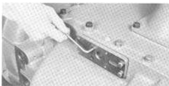
2. Install gasket and the air valve adapter plate. This takes two x-8-425 caoscrews, and two x-8-410 capscrews with x-3-400 washers. Make sure adapter plate is perfectly aligned with bore in case.
