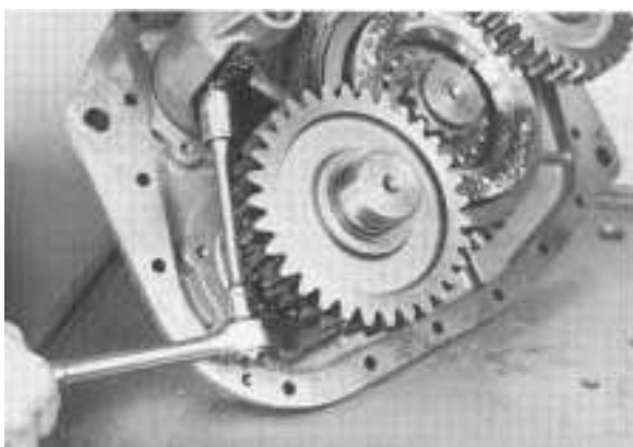
6. Install yoke lock screws, tighten and wire securely. Correctly position cylinder and install capscrews which attach cylinder to rear plate.
