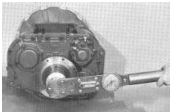
6. Lock transmission by engaging two gears with the sliding clutch gears; install flange or yoke on splines of output shaft and secure with nut, using correct torque of 450-500 ft.lb..
