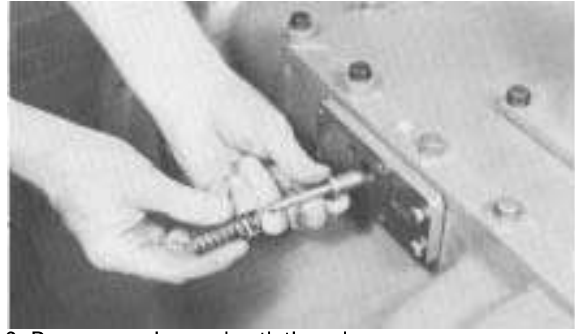
9. Remove spring and actuating pin.
