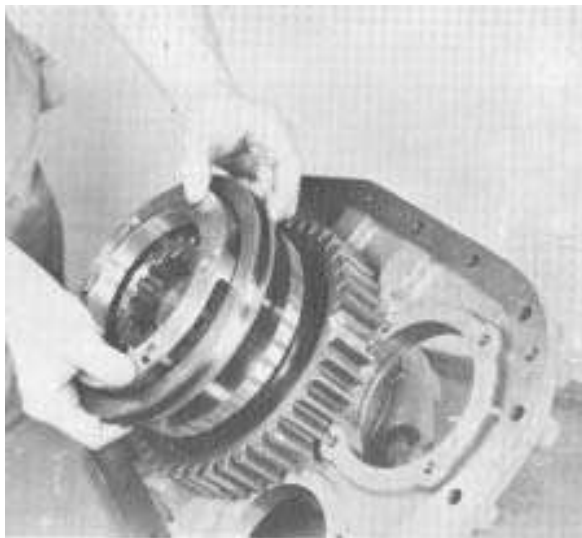
1. Remove synchronizer assembly from output shaft as a complete unit.
