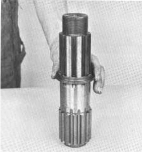
1. Install stepped washer on auxiliary mainshaft.
