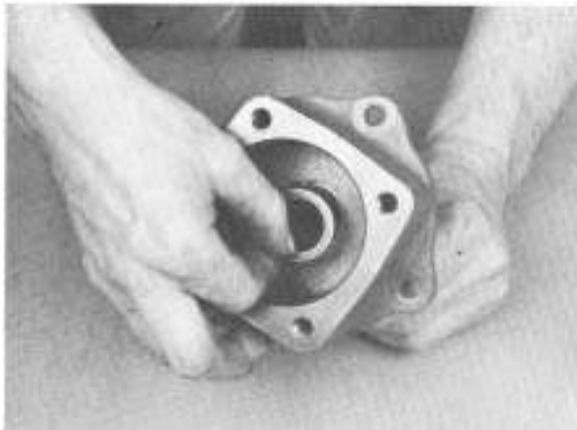
2. Install washer in shift cylinder against O-ring.
