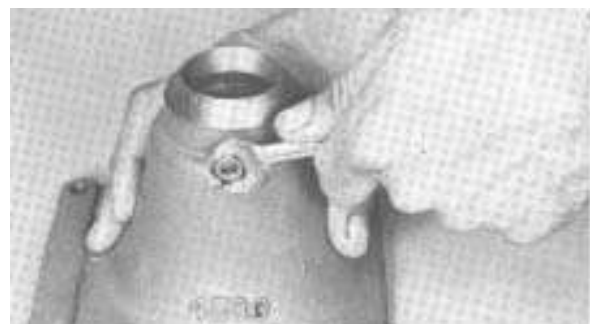
4. Remove nut and pivot pin if necessary.
