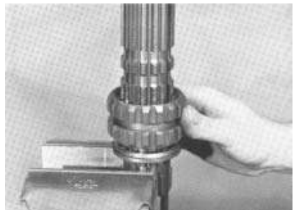
3. Install the first-reverse sliding clutch on shaft.
