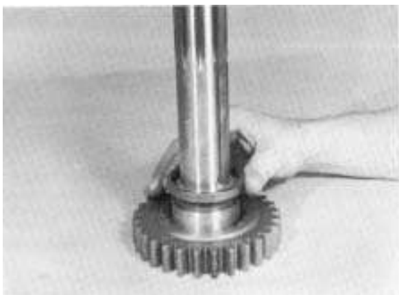
3. Install spacer on shaft.
