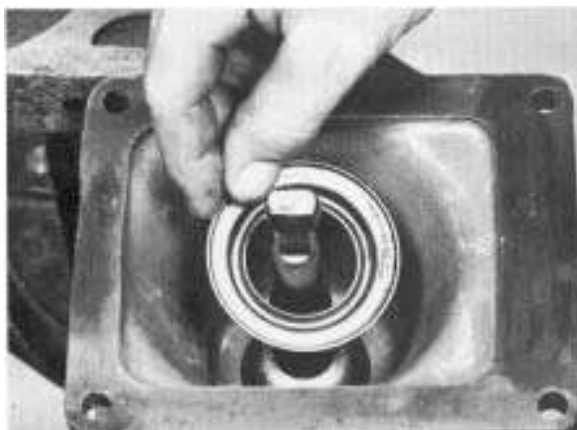
3. Place the tension spring washer in housing.
