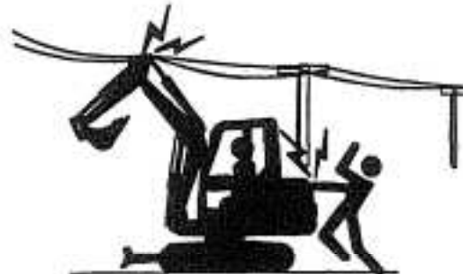
Electrical shock / electrocution
