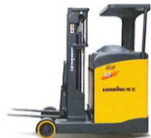
LG20DR OW:3415KG RP:2000KG B:48V/480AH LxH:2480*2601MM
