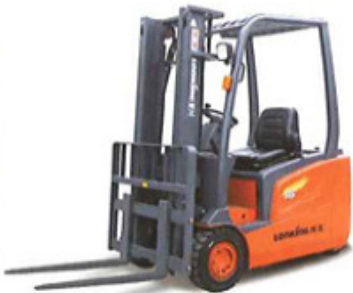
LG16B OW:3120KG RC:1600KG B:48V/480AH LxH:3018*2135MM
