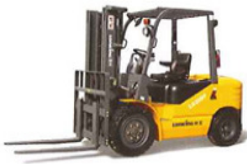
LGM300DT OW:4350KG RP:40KW RC:3000KG LxH:3775*2100MM
