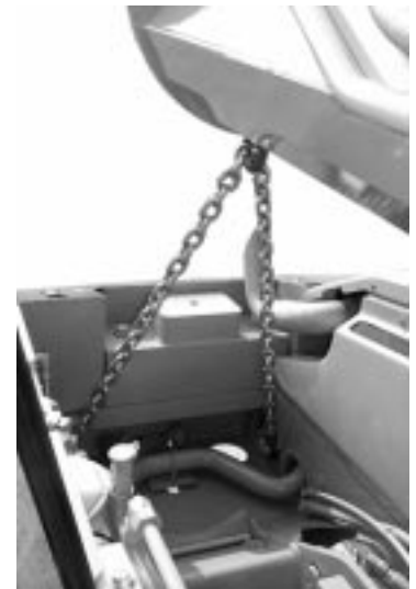
Figure 15-3 Boom Tie-Down Chain Installation
