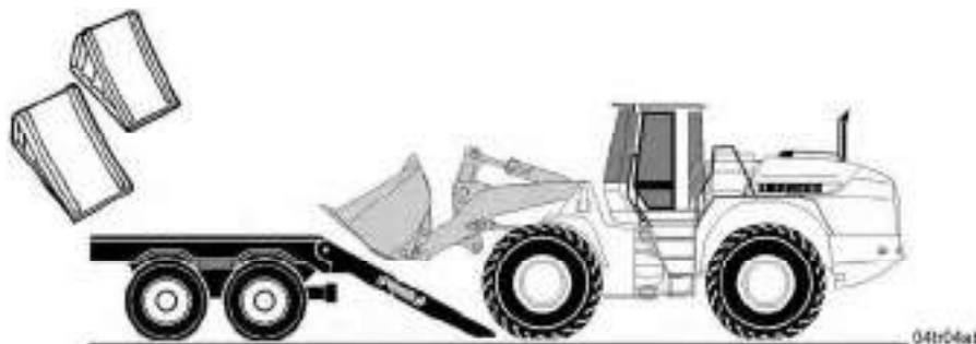
Loading the machine
