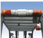
High Mounted Rear Combination and Beacon Lights
