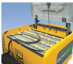
72V battery & AC traction for longer hours of operation
