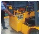
Easy Side removal of battery (optional)
