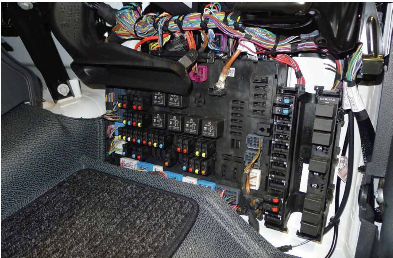
Location of SSAM in the electronics compartment on the passenger side
