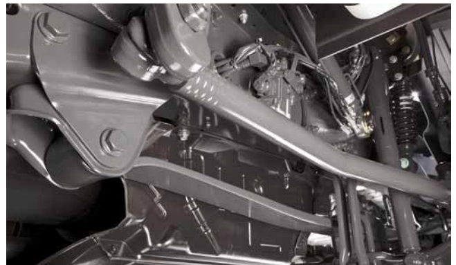
Front spring, 3.6 t, parabolic (Q1J)
