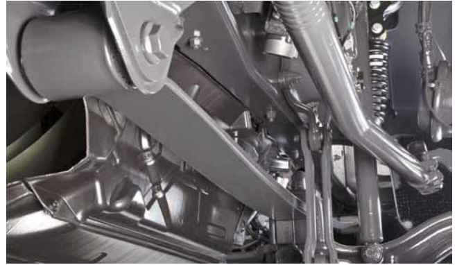
Front spring, 3.4 t, parabolic (Q1C)
