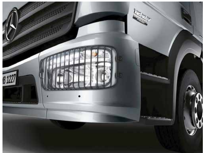
Stone impact protection, metal, for headlamps (L4Z)
