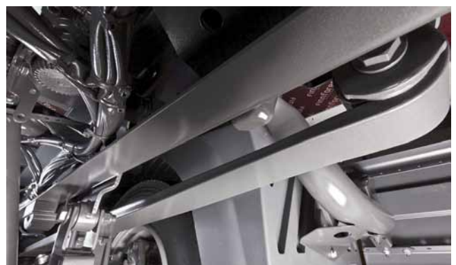
Rear spring, 5.0 t, parabolic, 1-leaf (Q2N)
