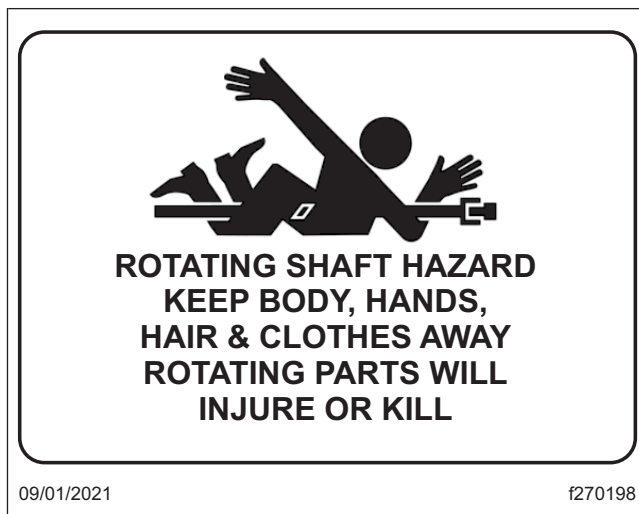
Fig. 1.1, PTO Safety Hazard Sign
