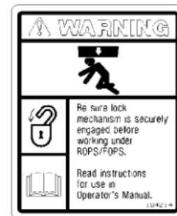
184214 – Located next to jack
